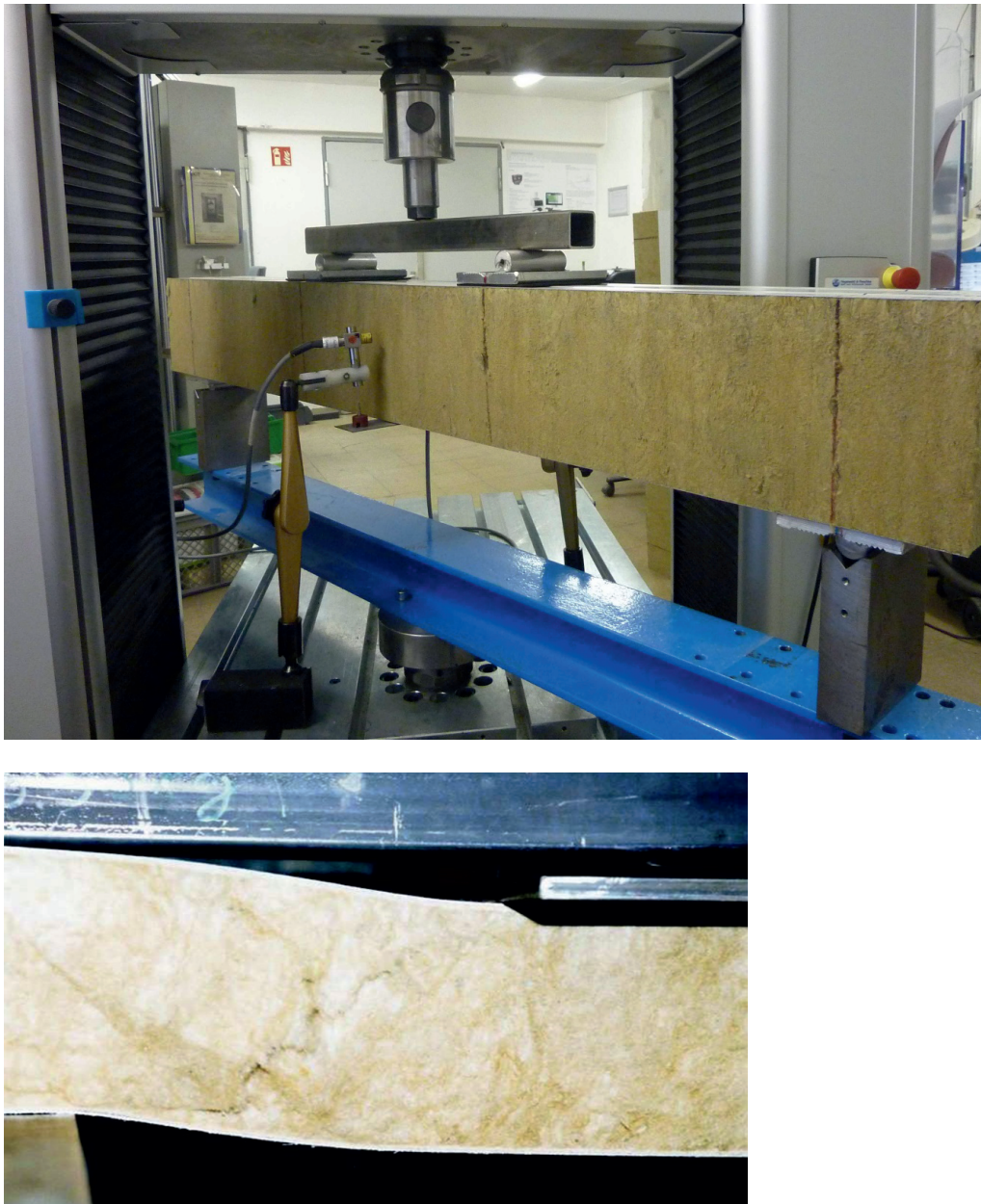
Figure 7: Shear tests on short beams of MW cored panels
