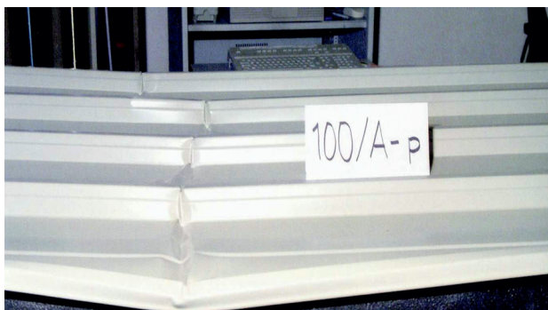
Figure 21: Buckling of the trapezoidal face (positive orientation)
