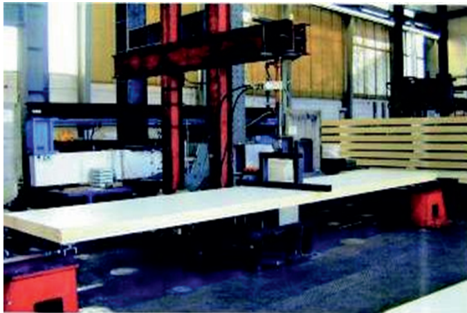
Figure 24: Internal support bending test with regular loading
