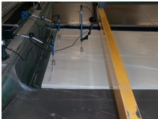
Figure 33: Test arrangement when using a vacuum chamber in support reaction tests
